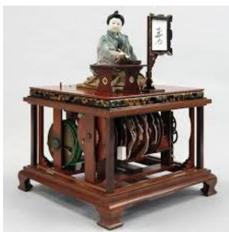
(Giumon`s machine doll, above doll moving, under part is machine block for above doll moving)
